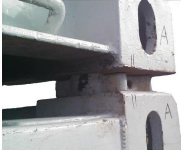
Figure 12. Containers Stacked on Connection Device (HEDD engineered design, n.d.).
